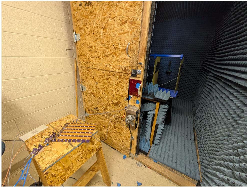
Figure 35. Receiver chain setup. A signal generator (left) feeds an LNA that drives the first column of the Blass matrix board. The first four beam outputs are downconverted and sampled using a Xilinx ZCU208 RFSoc board.
